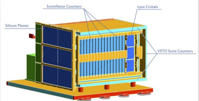
FIGURE 2. A schematic draw of the High-Energy Particle Detector: - in blue, the silicon tracker; - below the tracker there is the trigger plane (not seen here); - in light blue 16 plastic scintillators of the upper calorimeter; - on the right are visible three of the LYSO cubes of the lower calorimeter; - around the calorimeter three counters of the VETO can be seen; - in green the power supply and electronics.
