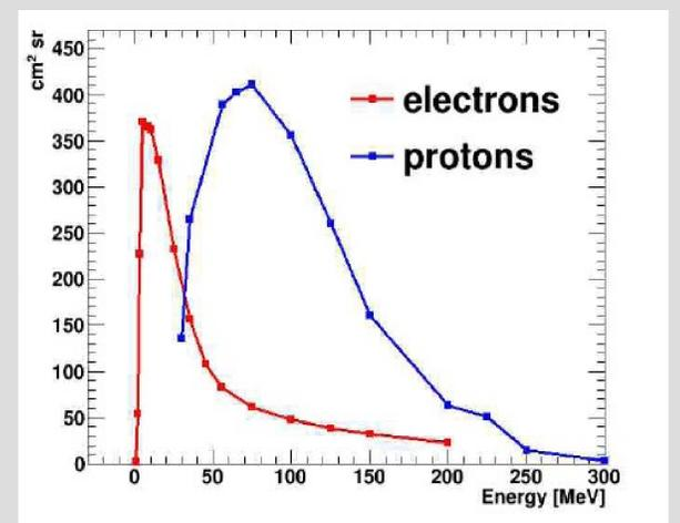
Figure 3: Expected acceptance for electrons and protons [3].
